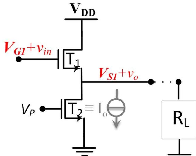
$$\begin{aligned}V_{out,max} &= V_{DD} - V_{DS,sat1} \\&= V_{DD} - (V_{gs1} - V_{Tp})\end{aligned}$$
