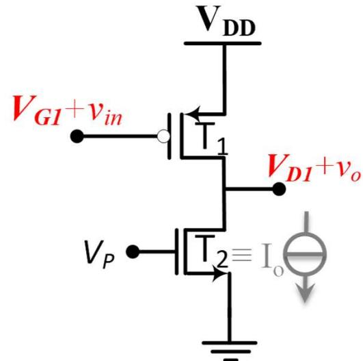
$$\begin{aligned}V_{out,max} &= V_{DD} - V_{DS,sat1} \\&= V_{DD} - (V_{sg1} - V_{Tp}) \\&= V_{G1} + V_{Tp}\end{aligned}$$
