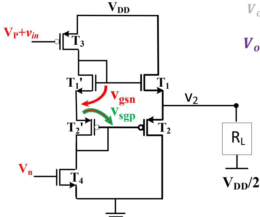
$$V_{out,max1} \approx V_{DD} - V_{DS,sat1}$$
